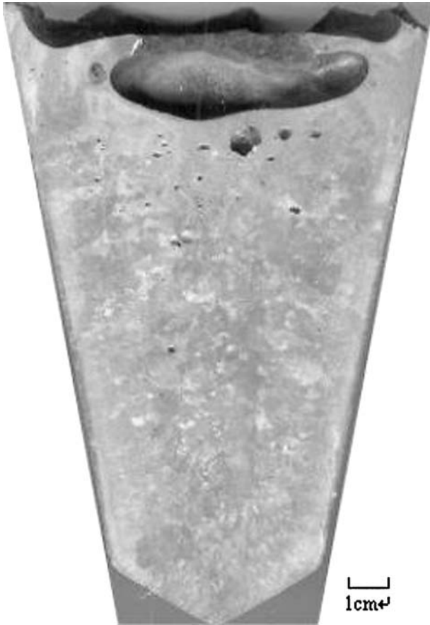
Figure 10 Experimental solidification grain structure of Ti-45 at%Al alloy ingot at the vertical section.
